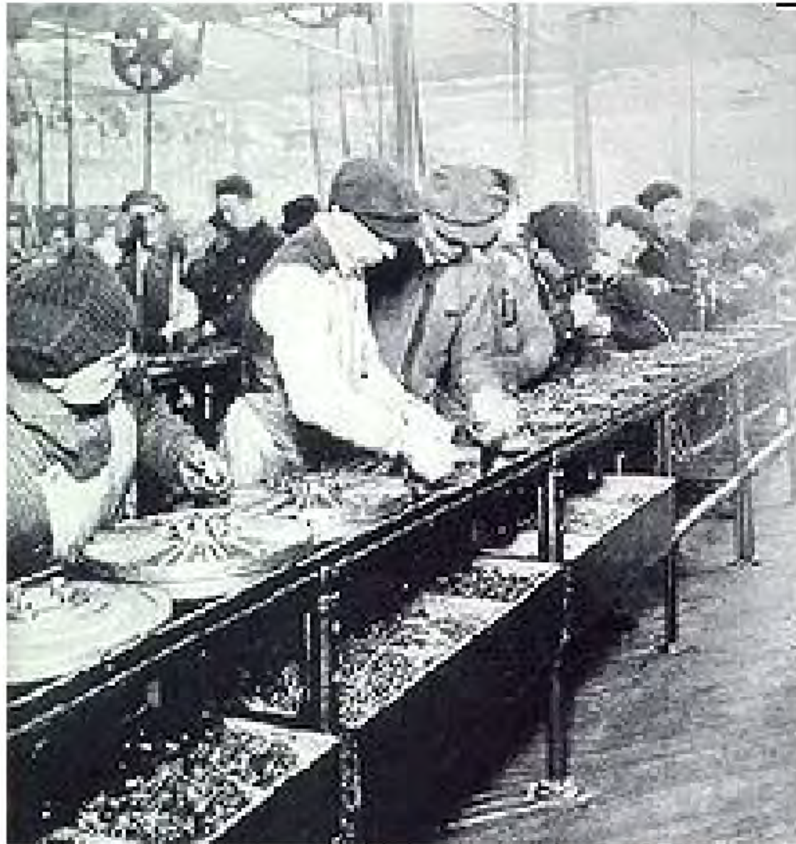
The first large-scale mass production assembly line at the Ford Motor Co. - the magneto assembly line in 1913
